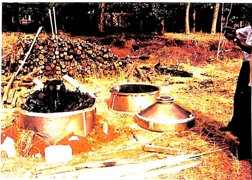
Photo 8 Taking out produced charcoal (A case of double-column system)
